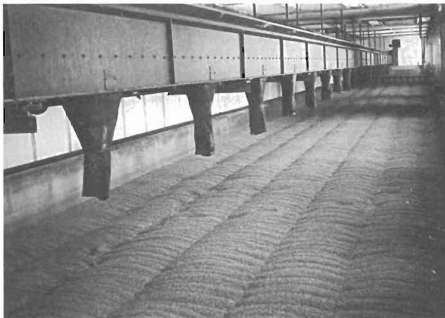
Forever waves of grain! Temperature, air flow and the mechanical turning of the green malt are carefully controlled in the malt house. A germination and kilning room is shown here.
