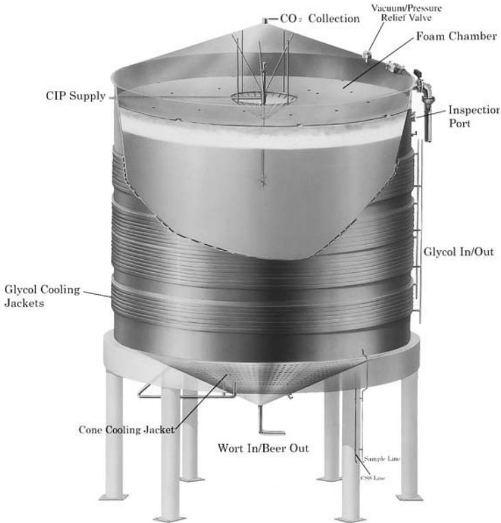
Figure 7.5 A schematic drawing of a cylindroconical fermentation vessel. Courtesy of Anheuser-Busch, Inc.
