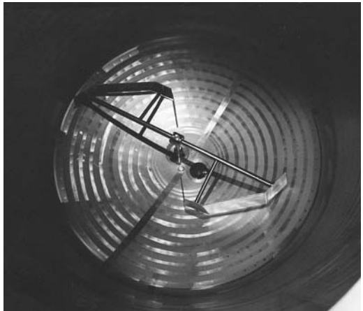
Figure 6.3 Inside a mash conversion vessel. The agitator is designed to ensure efficient and homogeneous mixing. Courtesy of Briggs of Burton.
