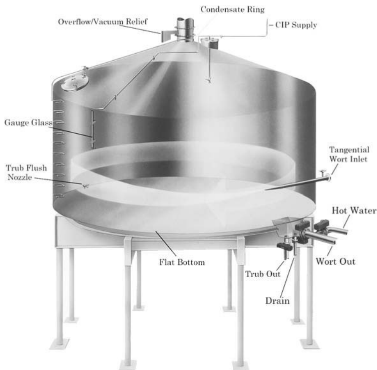
Figure 6.8 Diagram of a hot wort receiver ("whirlpool"). Courtesy of Anheuser-Busch, Inc.
