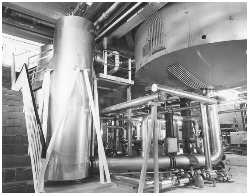
Figure 6.6 A kettle (right) with external calandria (left). Courtesy of Briggs of Burton.
